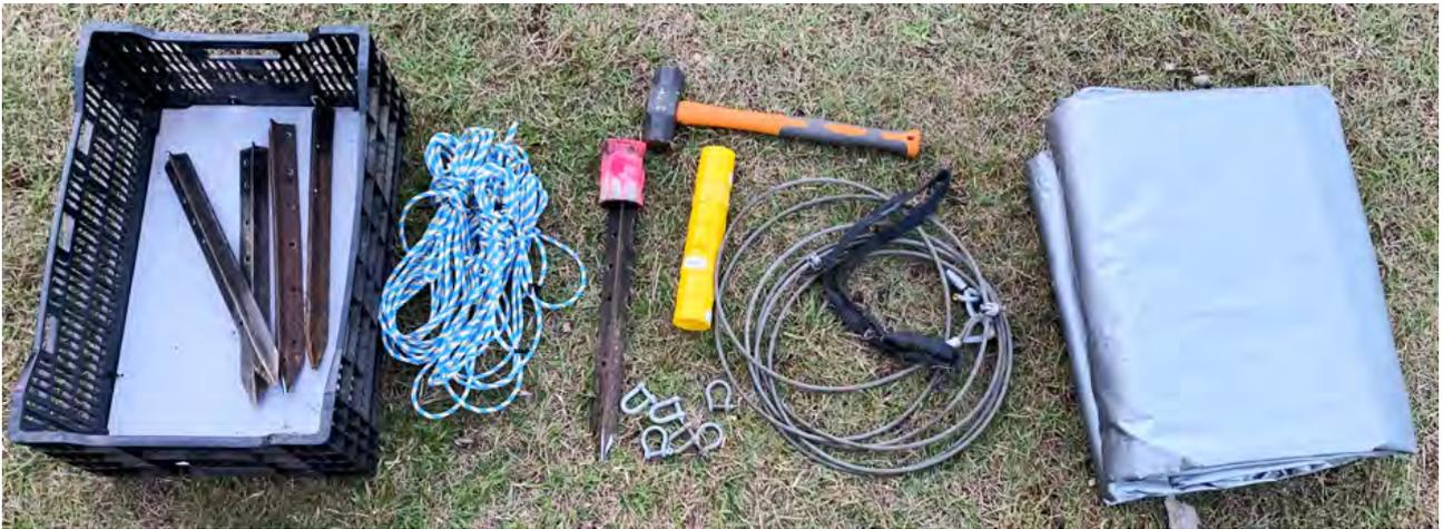
Take the steel cable (with sling and shackles) onto the roof and undo. Pay attention to how it was rolled up, so as to store it the same way. Attach either end of the cable to the front and back corners, **opposite** of the side you are having the tarp.
